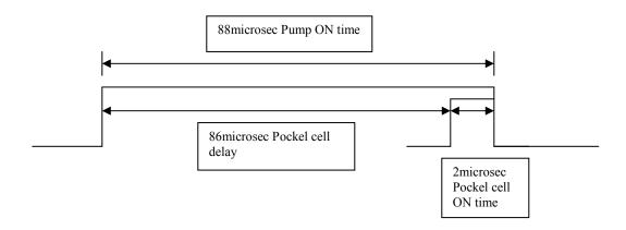
3. The Pump diode ON time can be increased to a maximum of 150microsec (minimum 50microsec) and the Pockel cell delay (minimum delay 45microsec) can be optimized between 100-150microsec to maximize the best output power.
