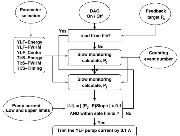
Fig. 4. A schematic describing the software feedback control.
