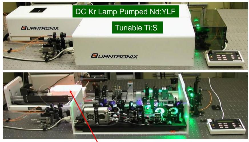
Ageing DC Kr lamp reduces laser pulse intensity, increases laser pulse width and timing.
