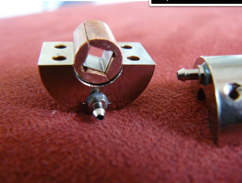
TiS LBO assembly (Lithium Triborate crystal, LiB 3 O 7 )
