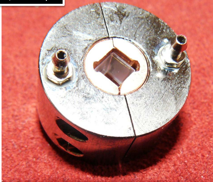
TiS LBO assembly (Lithium Triborate crystal, LiB 3 O 7 )
