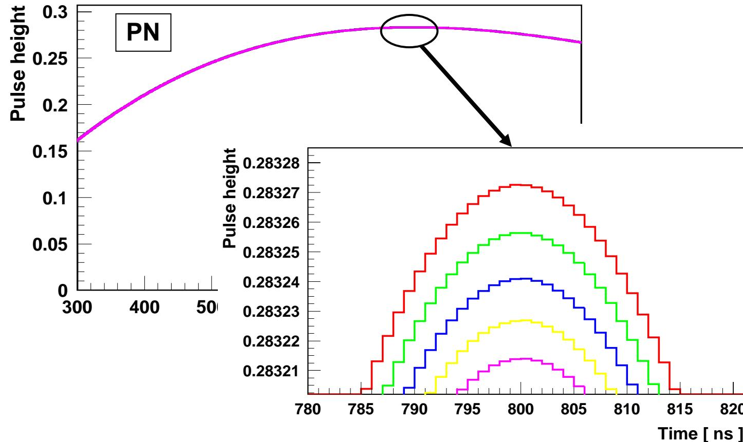
Because of the shaping time of the PNs the effect of the convolution is very small.
