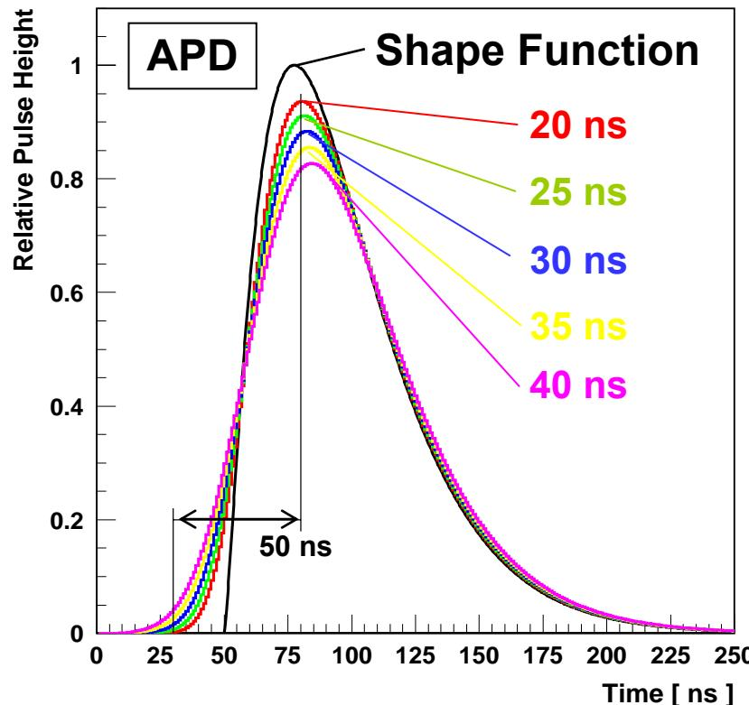
$$f(t) = \left( \frac{t - (T_{\max} - T_{\text{peak}})}{T_{\text{peak}}} \right)^{\alpha} \exp\left(-\alpha \times \left( \frac{t - T_{\max}}{T_{\text{peak}}} \right)\right)$$
