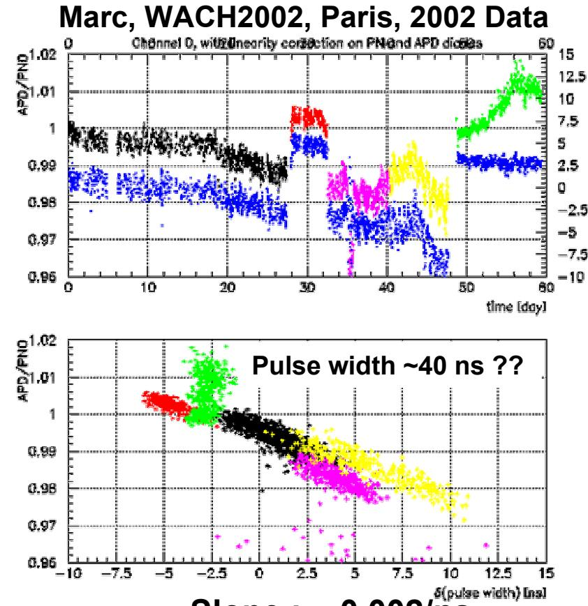
But : Pulse width determination different - From pulse rise time.
