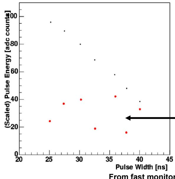
Attempt to compensate pulse energy change with the intensity regulator 'online' to isolate pulse width effect. Since pulse height non-linearity is much smaller this is not necessary.
