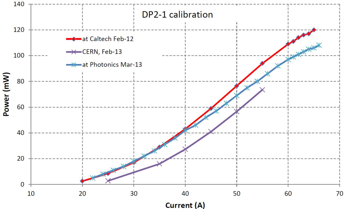
After replacing the THG crystal, the laser pulse energy met the specification of  $>1\text{mJ}$  at 62 A. It, however, is still lower than that after the delivery. Graham claims this is probably due to degradation of other parts in system, but so far no other part was found to be terribly wrong.
