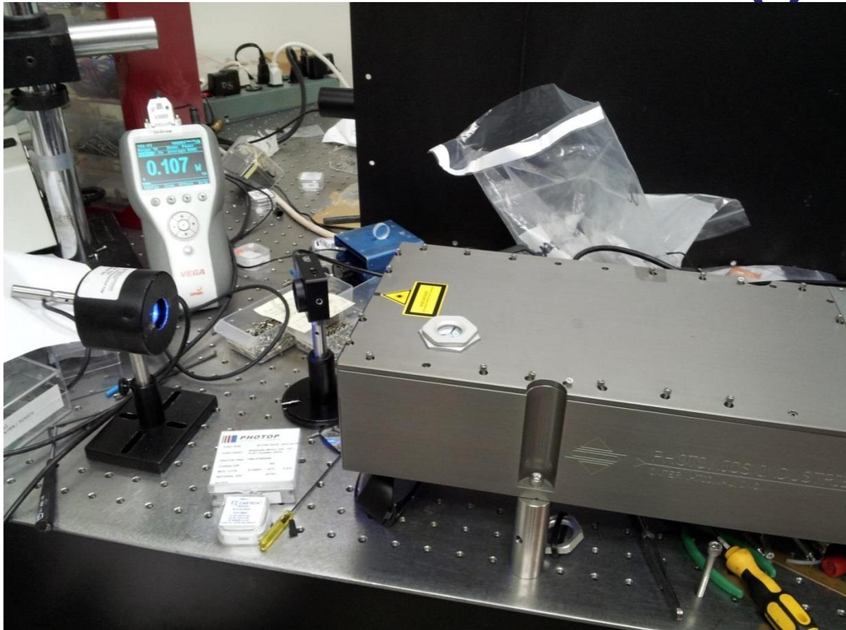
The cavity was checked at Photonics. The THG crystal was found to have a damaged coating. The coating was believed to be reliable, so this damage is probably an occasional incident. A new type of THG crystal, which is supposed to be more reliable, is installed and being tested. If it works, Photonics may also replace the THG crystal in the 2<sup>nd</sup> DP2.
