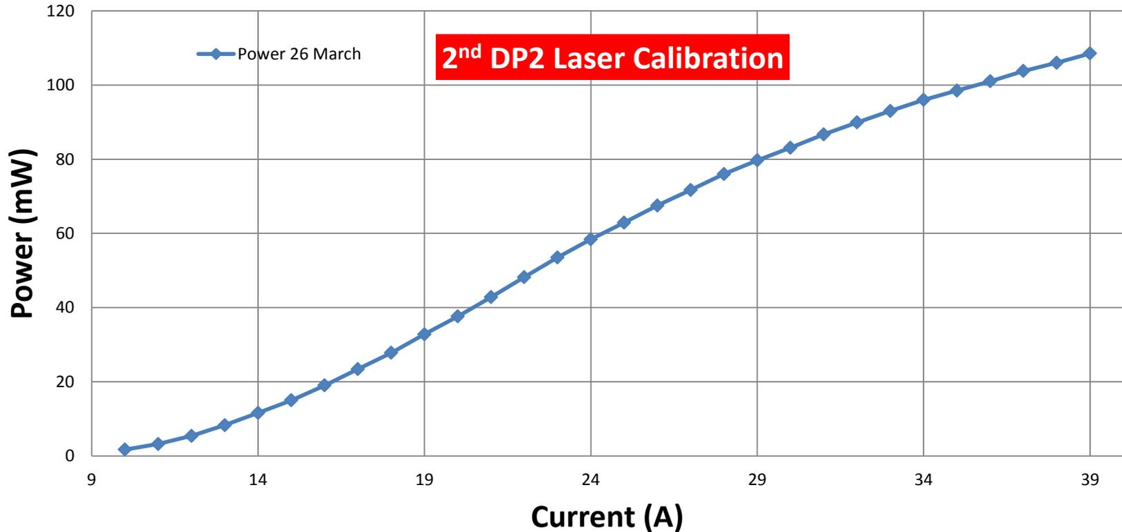
The Pulse energy meets the spec of 1 mJ at 36 A pumping current, indicating that the conversion efficiency from diode to laser pulse at 447 nm is ~1.8x higher than that of the 1<sup>st</sup> DP2. An explanation given by Photonics is that the emission wavelength of the pumping diodes in the 2<sup>nd</sup> DP2 has a better matching with the laser crystal absorption band. Further investigation is needed to fully understand this difference.
