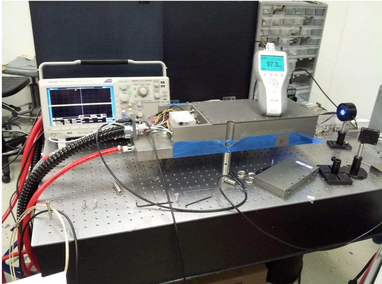
The construction of the laser head is finished. A commercial chiller with both heating and cooling functions was ordered but not yet delivered. The system tested has a temporary chiller.
