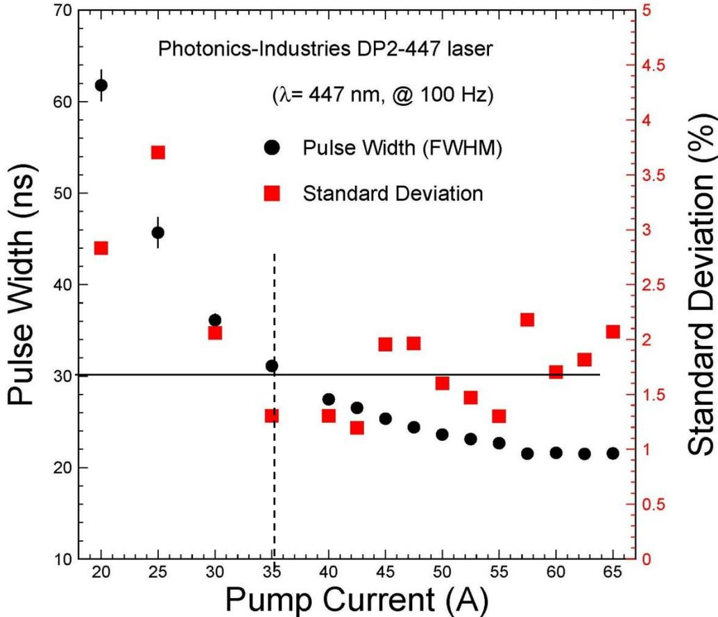
Above 35 A, the pulse width meets the spec:  $< 30 \text{ ns}$  with its instability about 2%.
