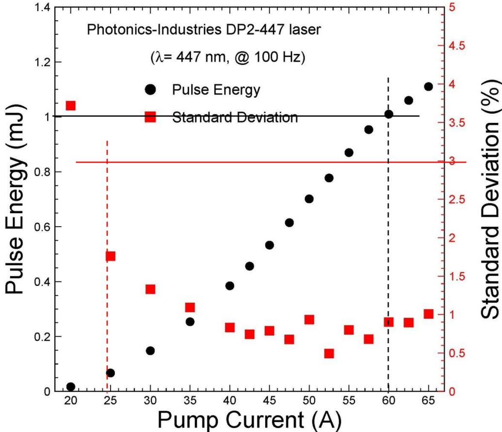
To reach 1 mJ pulse energy the pumping current should be  $\geq 60\text{A}$ .
