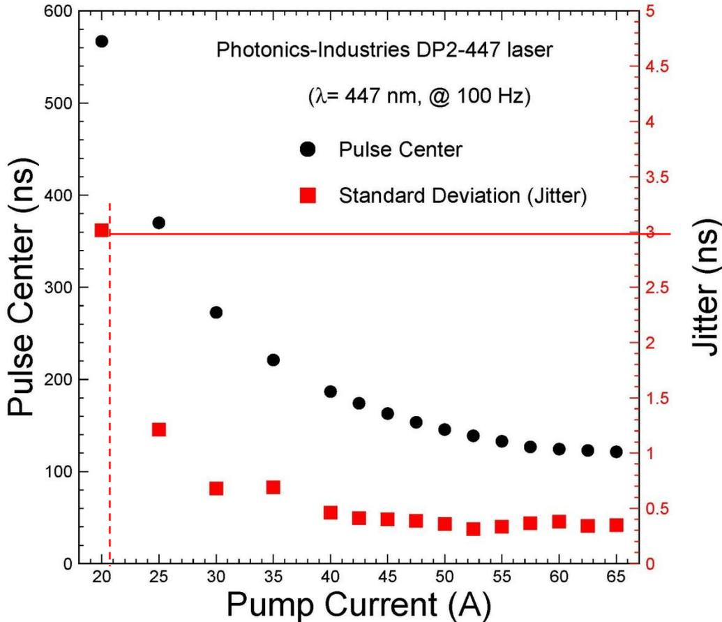
This laser featured with very small jitter of  $< 0.5 \text{ ns}$  for pumping current of  $> 40 \text{ A}$ .
