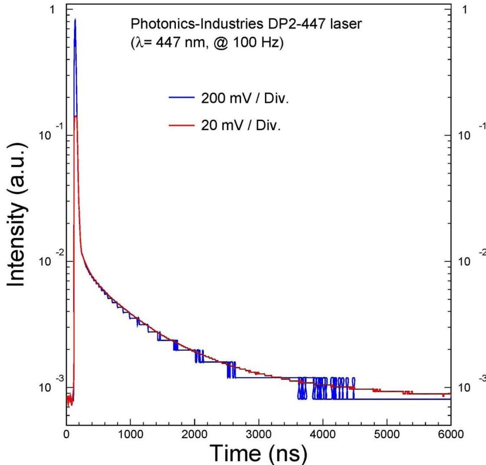
At 60A pumping current, the laser pulse was measured at two scales by using an average function of the DSO (256).
