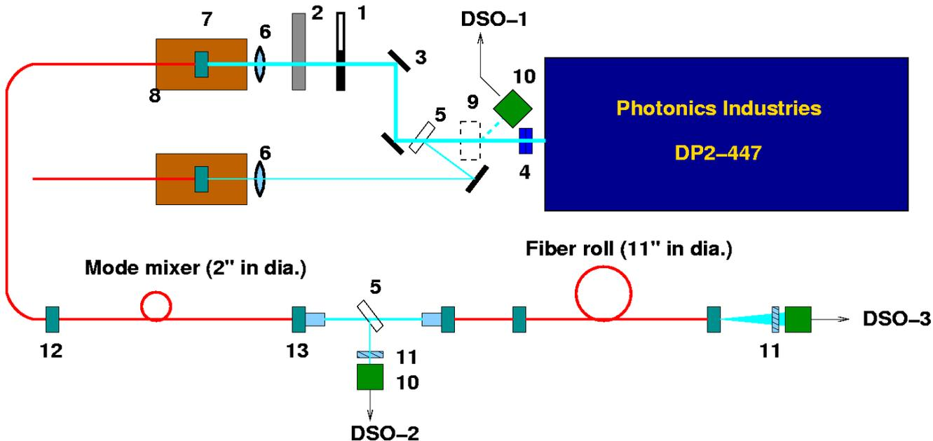
DSO-2 and 3 were used to measure fiber dispersion
