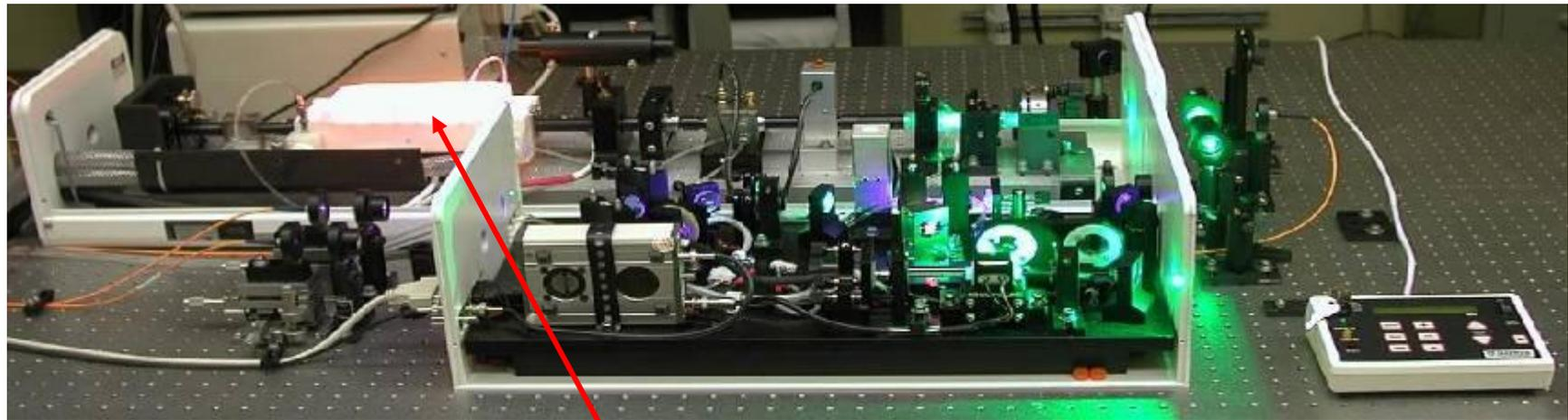
Ageing DC Kr lamp reduces laser pulse intensity, increases laser pulse width and timing.
