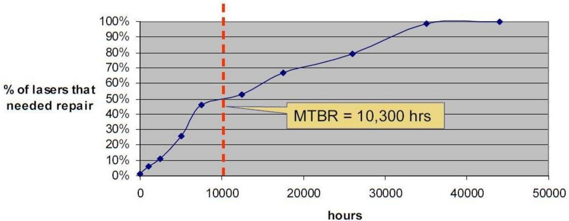
MTBF is at 10,000 h for Diode pumped solid state lasers
