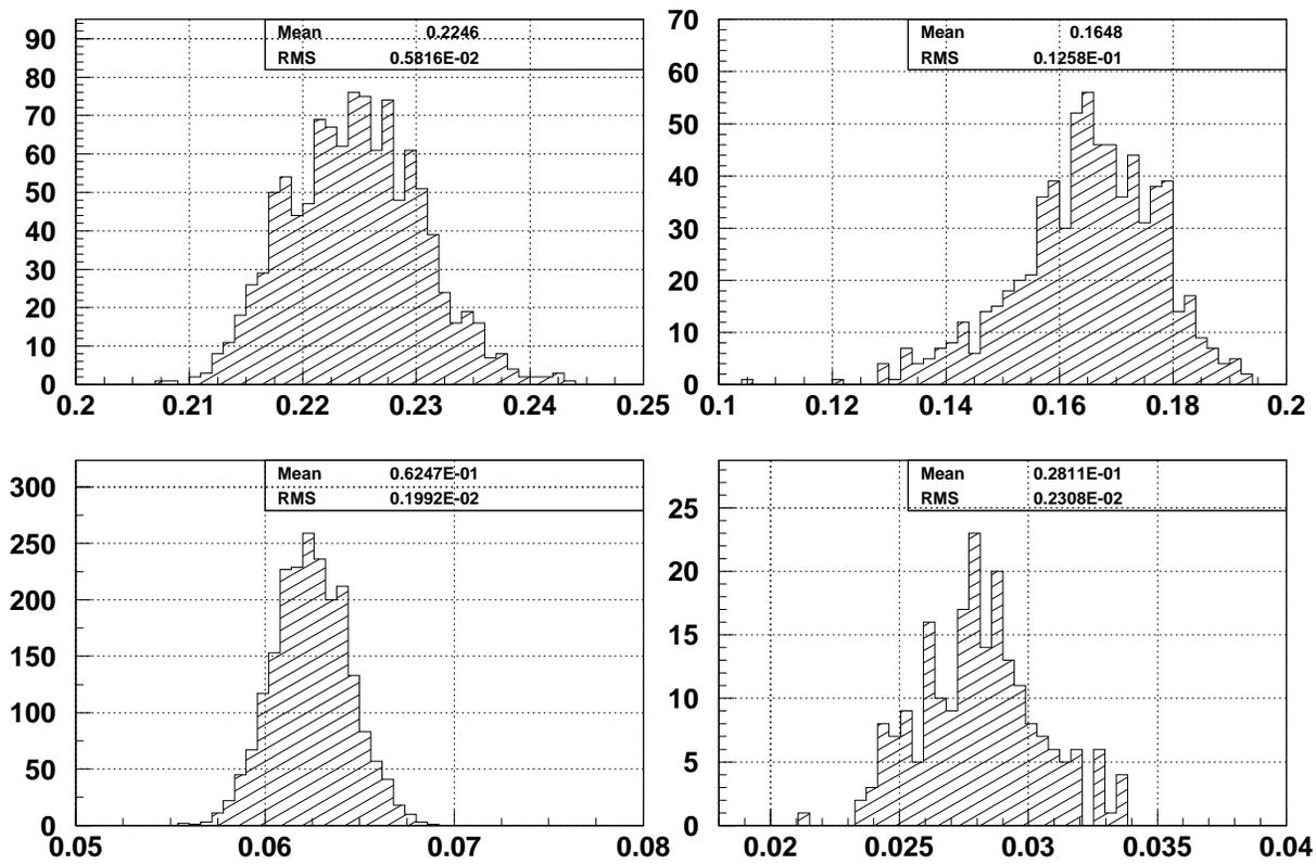
Figure 7: Distribution of laser pulse energy obtained in 25 hours for four wavelengths.
