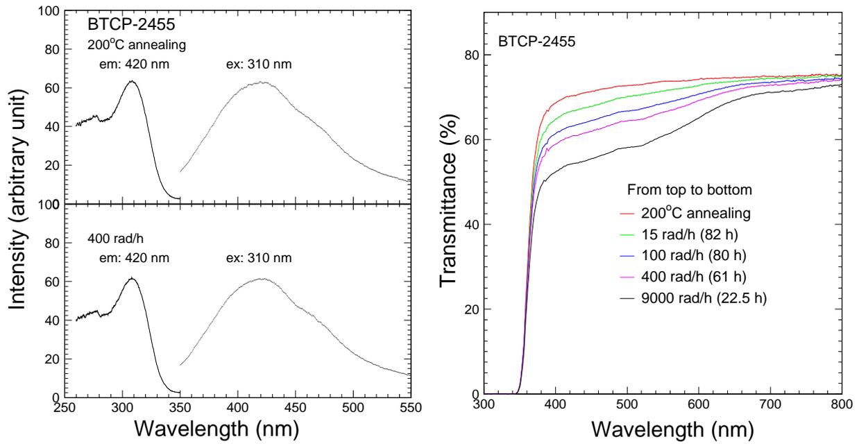
Figure 1: The excitation and emission spectra before and after irradiation at 400 rad/h (left) and the transmittance spectra at equilibrium under irradiations of several dose rates (right) are shown as function of wavelength for a PWO sample.
