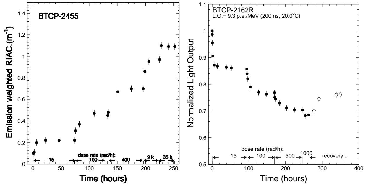
Figure 2: The damage history of the emission weighted radiation induced absorption coefficient (RIAC, left) and the light output (right) are shown as function of time for two PWO samples.
