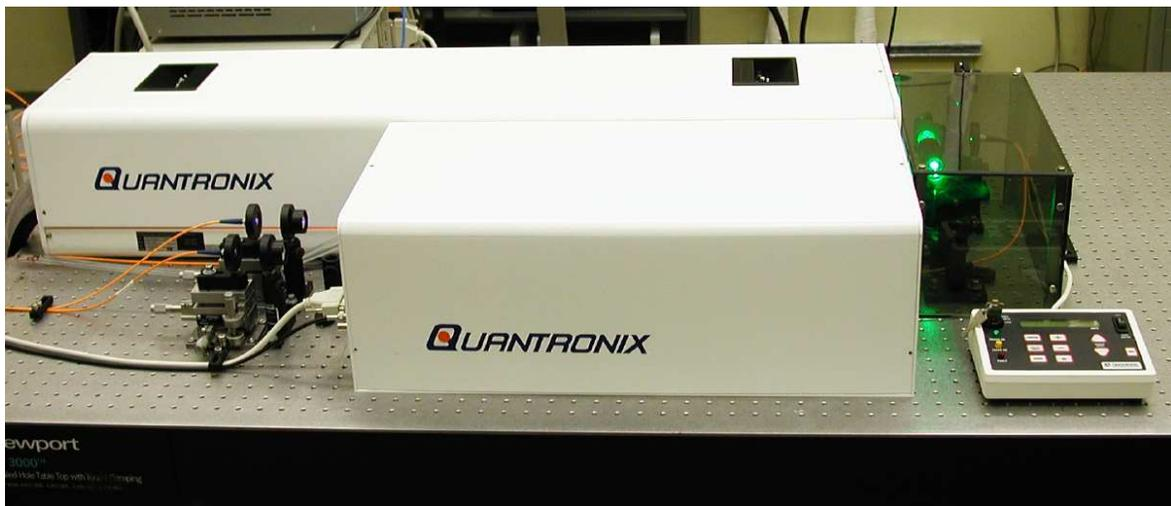
Figure 4: A photo of the Quantronix laser system showing the Nd:YLF pump laser (back) and the tunable Ti:S laser (front).
