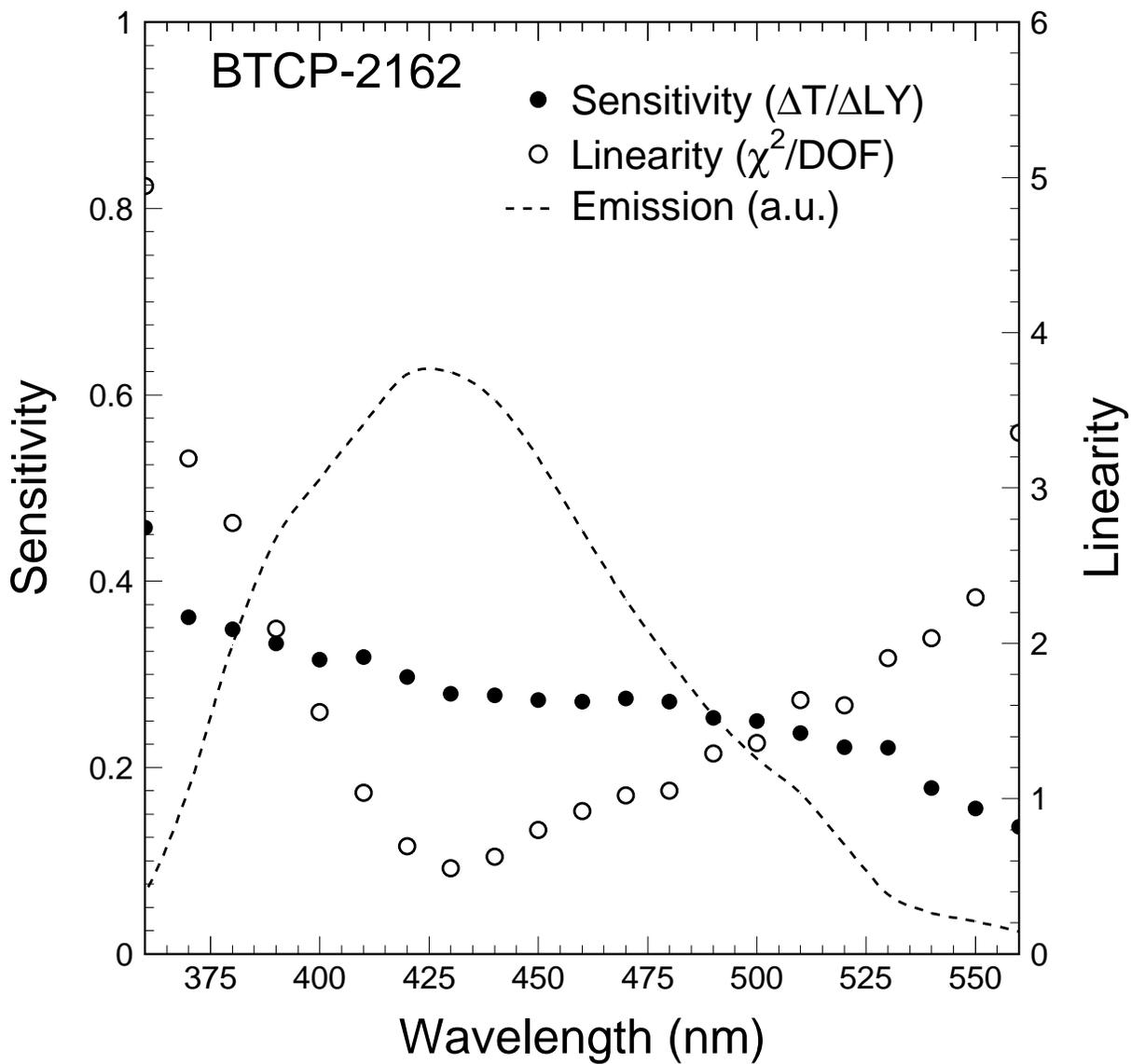
Figure 5: Monitoring sensitivity, linearity and emission spectrum are shown for a PWO sample.
