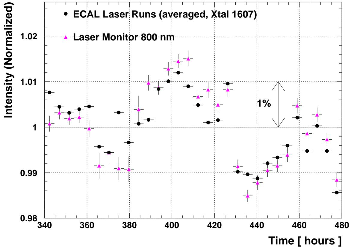
Figure 9: A comparison of laser pulse intensities measured in 6 days by ECAL APD readout (black) and laser internal monitor readout (red).
