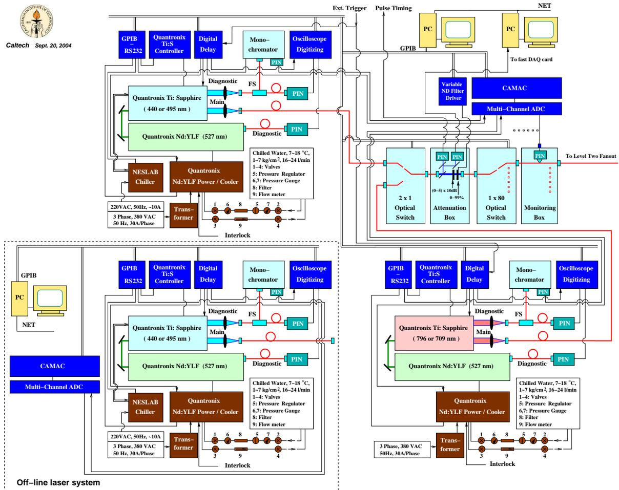
Figure 3: A schematic showing the design of the laser based monitoring light source and high level distribution system.
