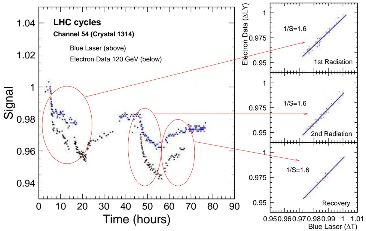
Figure 10: History of 120 GeV electron (black) and 440 nm laser (blue) data are shown as function of time during an irradiation beam test. Three expansions at right show the same linearity between electron and the monitoring signals.
