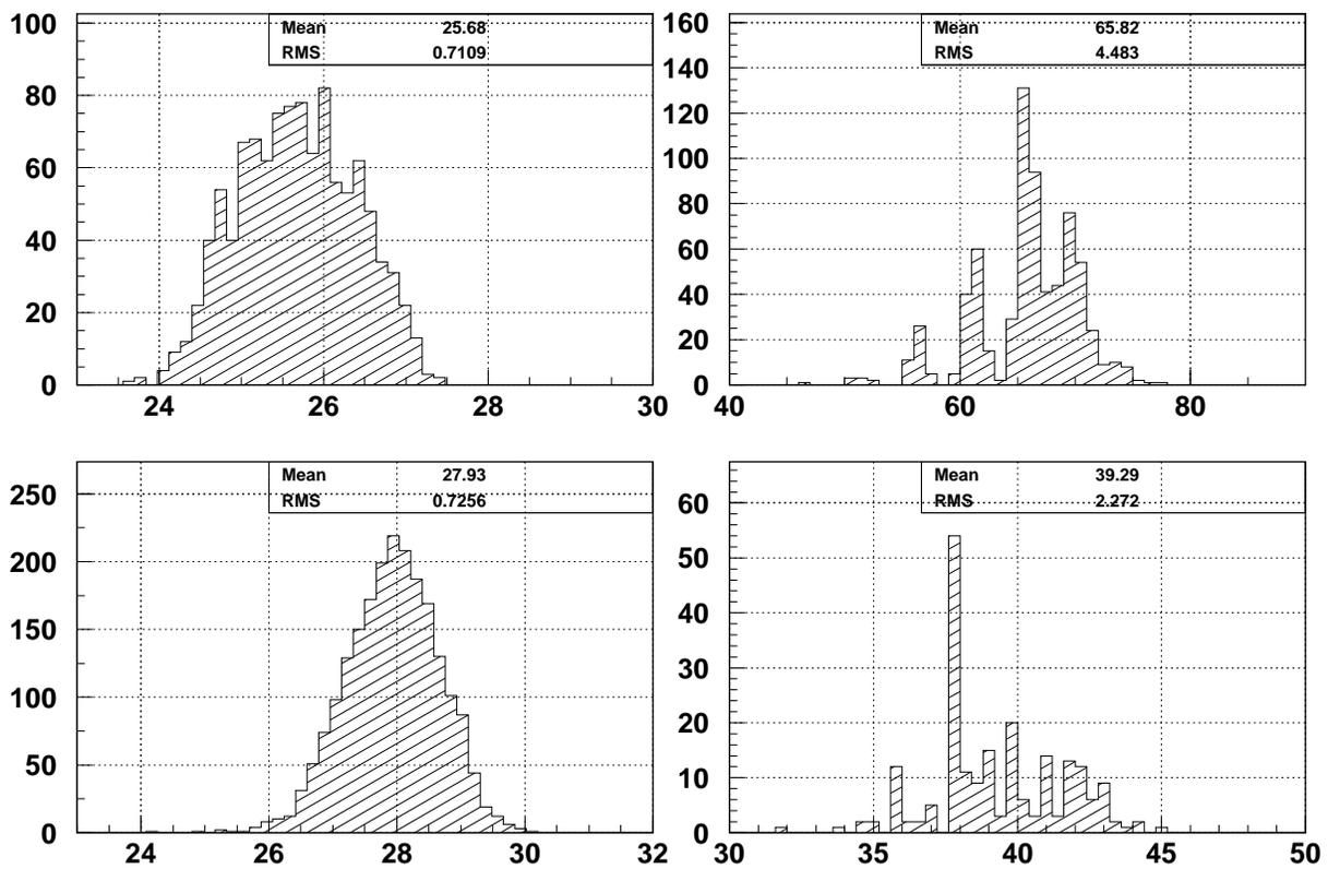
Figure 8: Distribution of laser pulse width obtained in 25 hours for four wavelengths.
