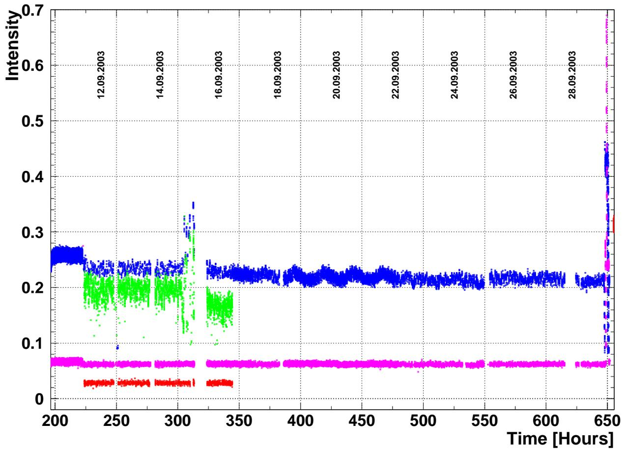
Figure 6: Laser pulse intensity is shown as function of time (h) during a 19 day period in a beam test at CERN, where blue, green, pink and red represent laser pulse energies at 440, 495, 709 and 796 nm respectively. Vertical spreads in the middle left (320 h) and right (650 h) are laser pulse energy scan runs for electronics test.
